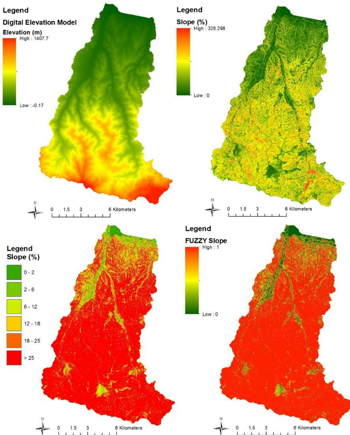
**Fig. 12: The DEM (a) used in order to calculate slopes (b) in Tavronitis basin. The Spatial distribution of reclassified slope values (c) and the results of fuzzy membership function application (d) are also presented**
