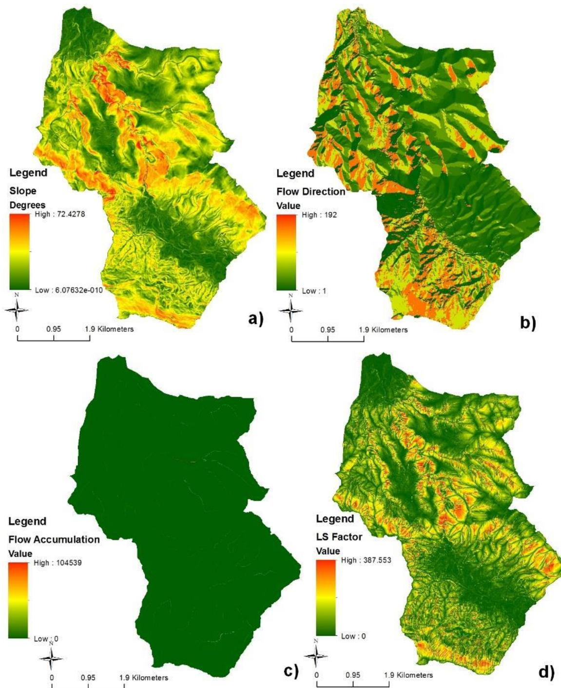
**Fig. 28: Spatial distribution of slope (a), flow direction (b), flow accumulation (c) and topographic (LS) factor (d) in Havgas - Milatos sub-basin**
