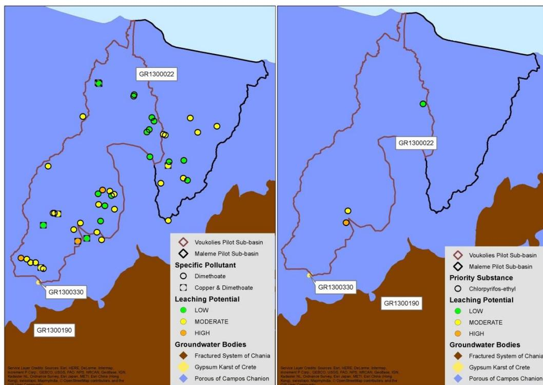
**Fig. 94: Spatial distribution of parcels where PPPs with specific pollutants (left) and priority substances (right) are used and classification according to their leaching potential in Voukolies and Maleme sub-basins**
