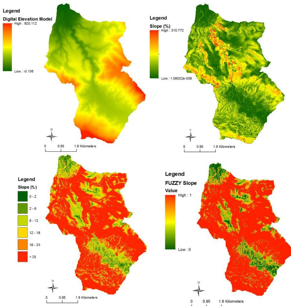
**Fig. 5: The DEM (a) used in order to calculate slopes (b) in Havgas - Milatos sub-basin. The spatial distribution of reclassified slope values (c) and the results of fuzzy membership function application (d) are also presented**
