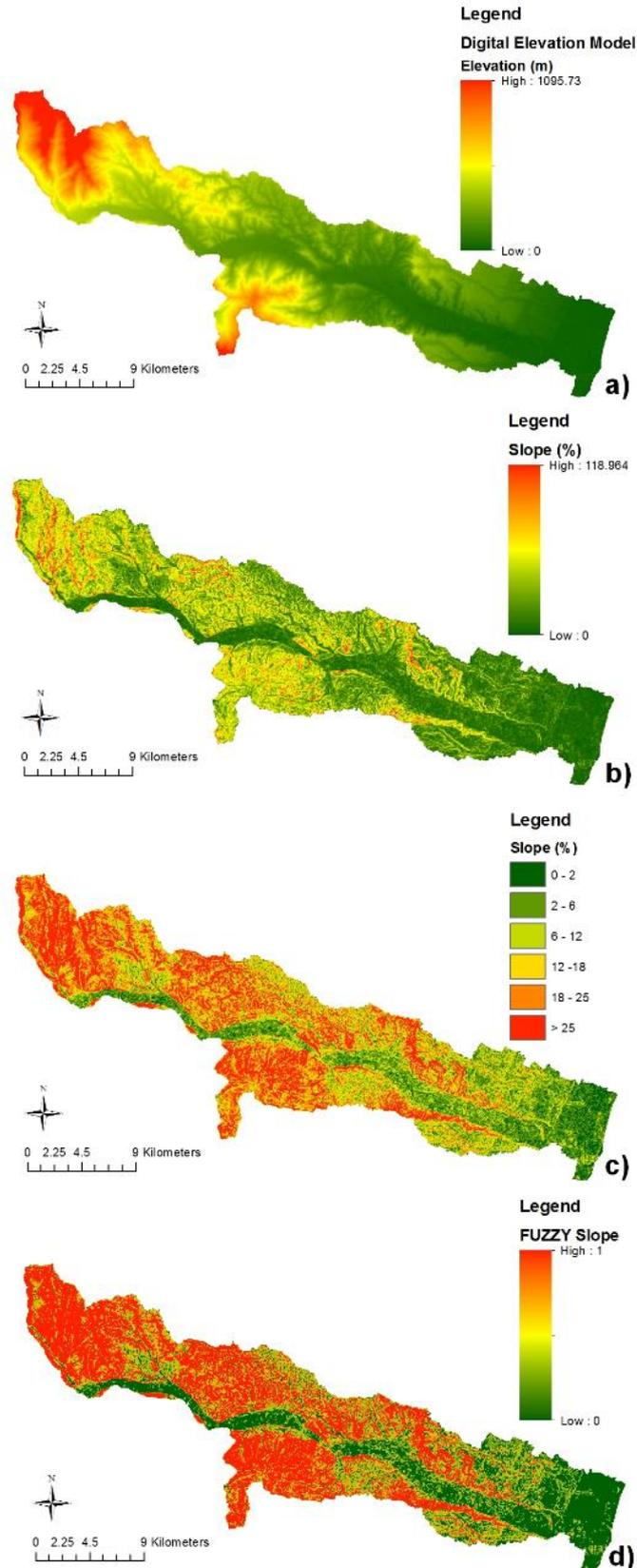
**Fig. 19: The DEM (a) used in order to calculate slopes (b) in Agri sub-basin. The Spatial distribution of reclassified slope values (c) and the results of fuzzy membership function application (d) are also presented**
