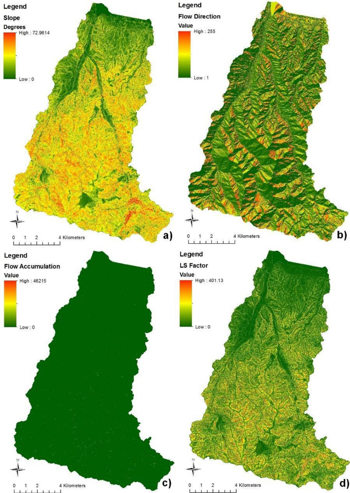
**Fig. 33: Spatial distribution of slope (a), flow direction (b), flow accumulation (c) and topographic (LS) factor (d) in Tavronitis basin**
